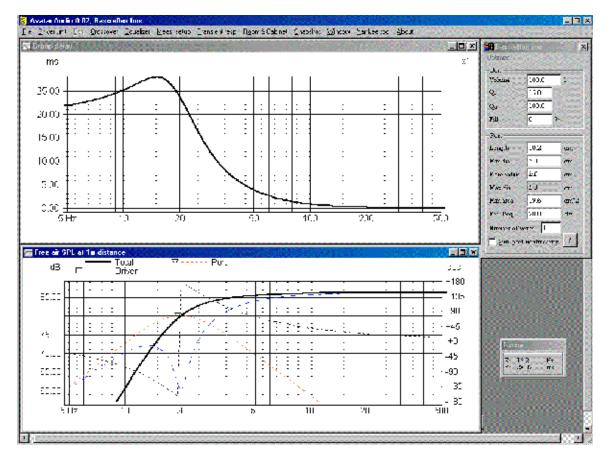
As we can see, the vented response shows the classic "phase wrap" at tuning, which is indicative of a higher order system. In fact, the vented system is a fourth order system, meaning that we will have a fairly steep transition from passband to fall-off.
