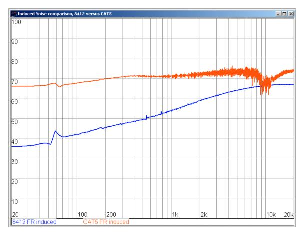
The blue line is for the 8412; the red line is for the CAT5. As we can see, the 8412 enjoys a healthy 10+ dB better rejection at all frequencies below 3 kHz; at the low end (100 Hz) there is over 26 dB better rejection of the induced currents/signal.
