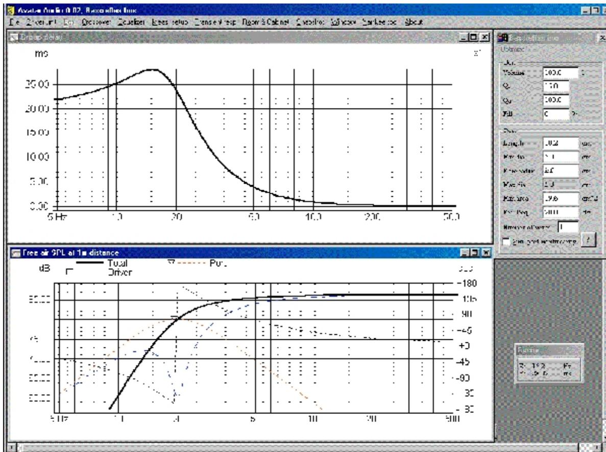
As we can see, the vented response shows the classic "phase wrap" at tuning, which is indicative of a higher order system. In fact, the vented system is a fourth order system, meaning that we will have a fairly steep transition from passband to fall-off. The group delay of the vented system peaks at 28 ms, at 15.2 Hz.
