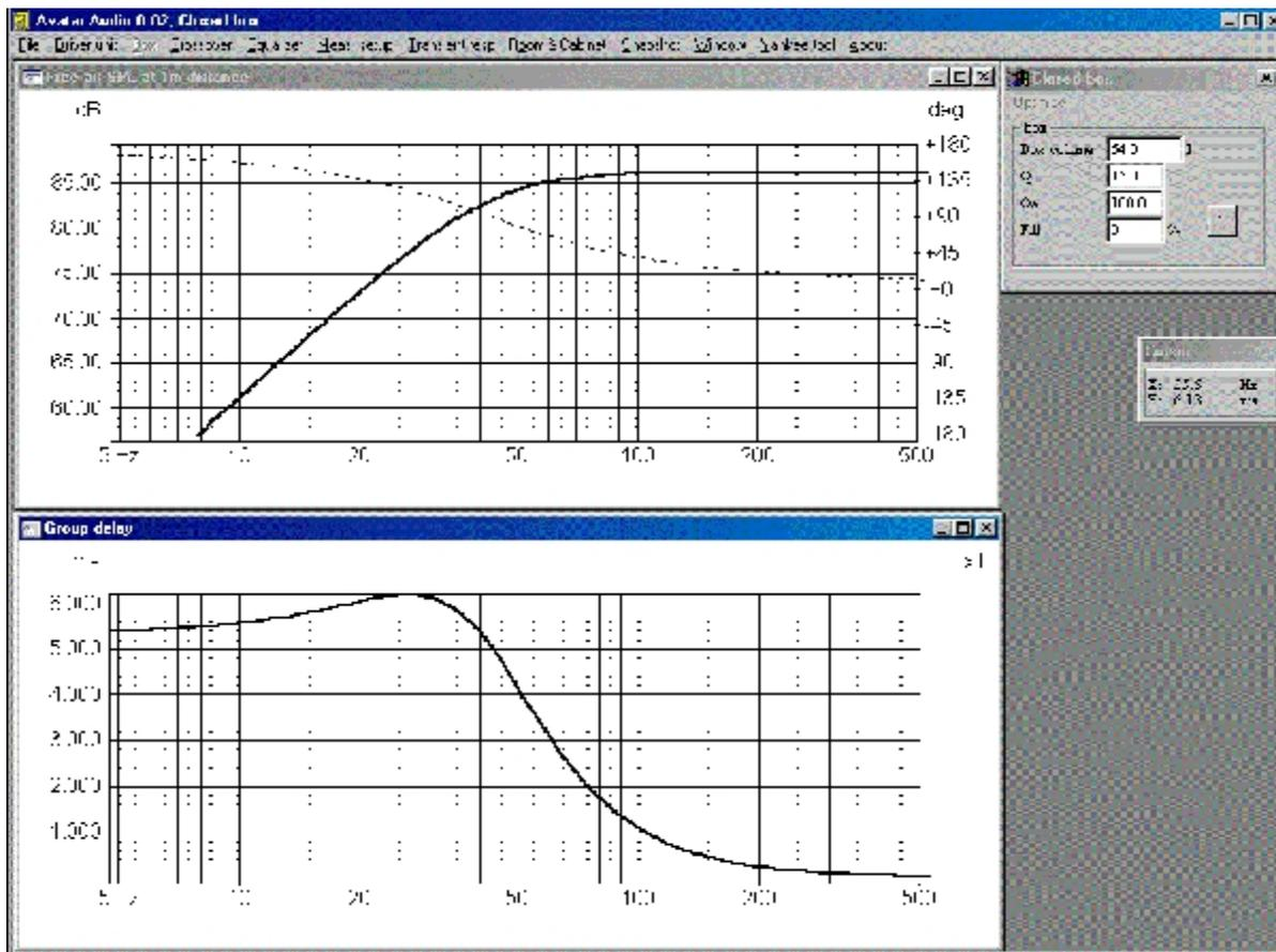
Here we see that group delay peaks at 6.13 ms . This is over 4 times better than the vented case, and over 5 times better than the passive radiator case. Given that a sealed box is a second order system, and as such does not exhibit a rapid fall-off on the low end (nor the attendant 360 degree phase wrap of the vented or passive radiator systems), the overall group delay will be considerably lower.
