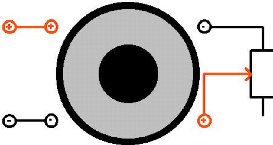
Adjusting the potentiometer to move the wiper towards the open end will increase the resistance seen by the second voice coil; adjusting the potentiometer the other way will decrease the resistance.
