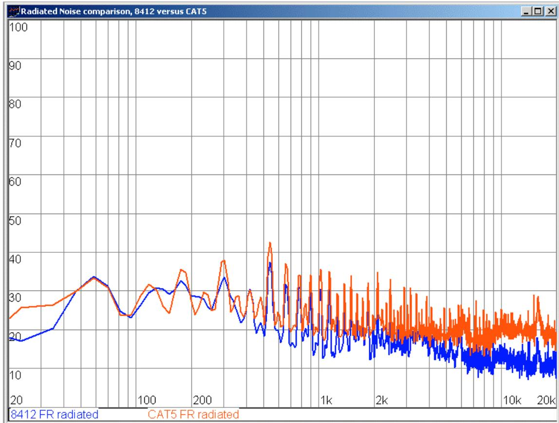
The blue line is for the 8412; the red line is for the CAT5. As we can see, the two cables are nearly equal down in the deep end of the spectrum (below 300 Hz). Above 300 Hz, the 8412 begins to show superior rejection of noise, and in fact in the top octave (from 10 kHz to 20 kHz) the 8412 has a solid 8-10 dB advantage in noise rejection, as compared to the CAT5.
