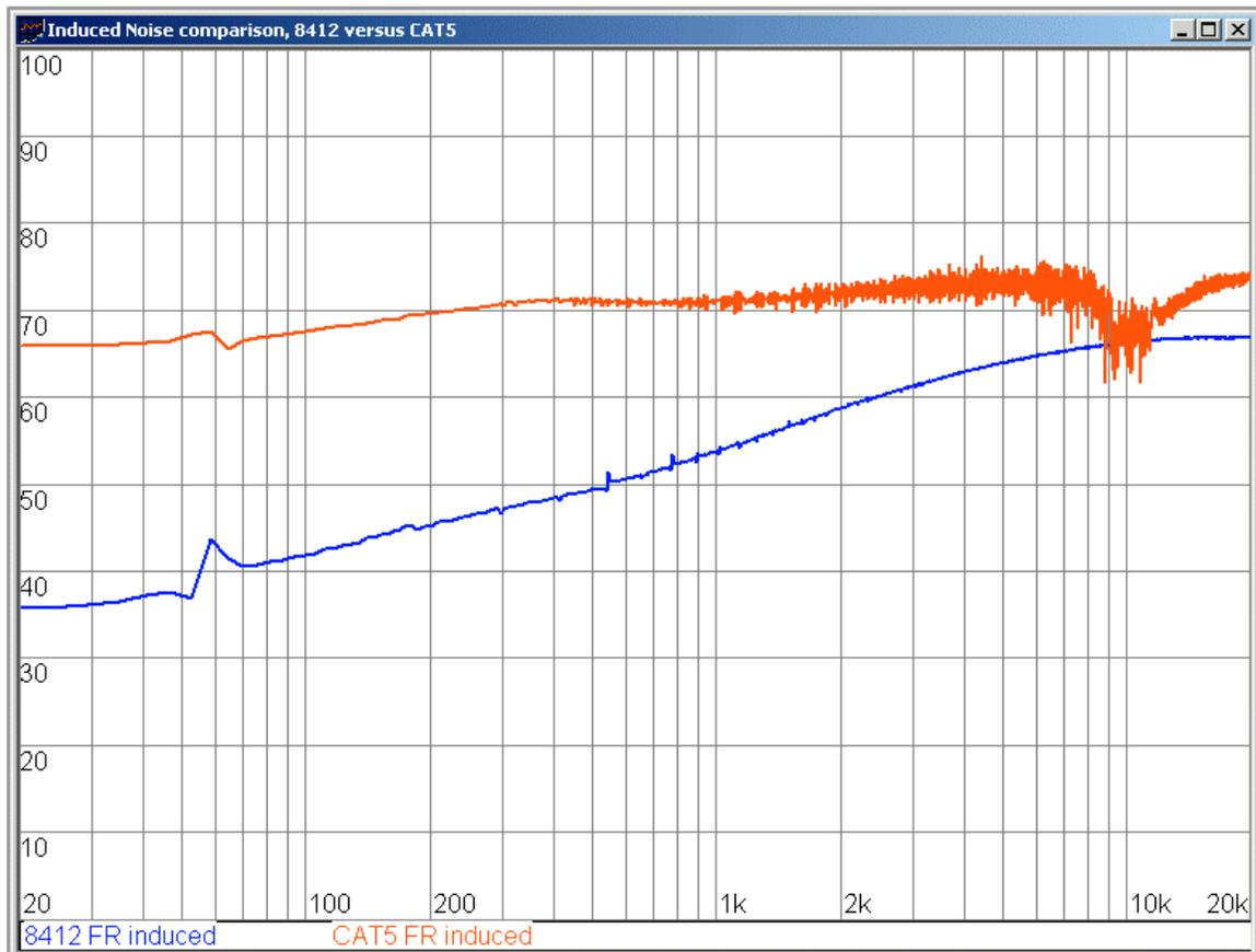
The blue line is for the 8412; the red line is for the CAT5. As we can see, the 8412 enjoys a healthy 10+ dB better rejection at all frequencies below 3 kHz; at the low end (100 Hz) there is over 26 dB better rejection of the induced currents/signal.
