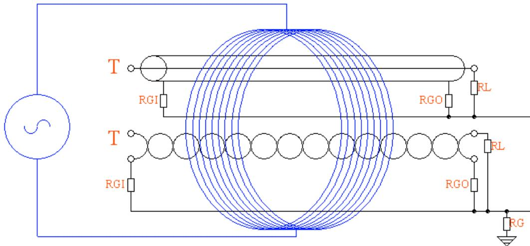
In this manner I was able to sweep a 20 Hz to 20 kHz signal into a magnetic field, then measure the induced signal pickup in the cable. I could get the rejection of the signal across all frequencies, and would get a measured "induced" frequency response of each cable.
