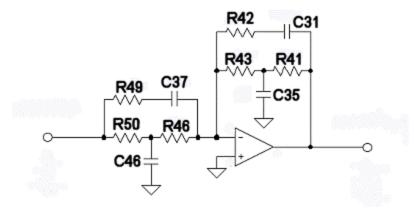
Thus you would stuff calculated values R1 into R50 and R46, calculated R2 values into R49 and R42, and so on.
