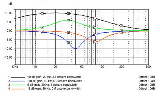
This graph shows just some of the functionality available with this type of EQ. The gain adjusts the peak level of the EQ (either boost or cut). The bandwidth adjusts the frequency range over which the EQ works. The Fc adjusts where the peak of the EQ happens.
