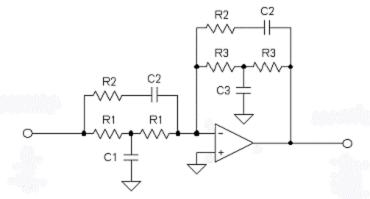
Calculate the standard R1/R2/R3/C1/C2/C3 values. The layout on the PCB uses the following schematic:
